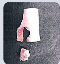
Results of Ti-Por ® push-out. Bone was fractured around the cylinder.
